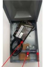
Plastic Electronics Case    IR Scope    Opening in Housing for Sensor
